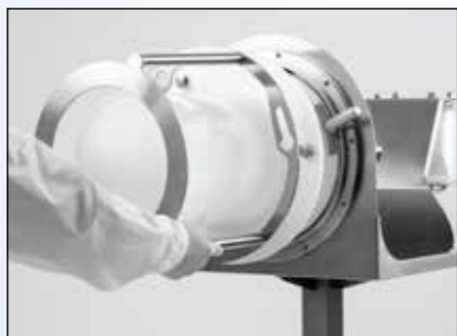
Remove the retention basket
