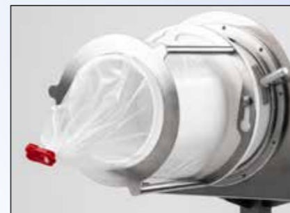
Close the continuous liner with SafeSeal
