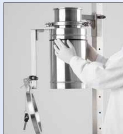
Fit the O-ring on the carrier tube
