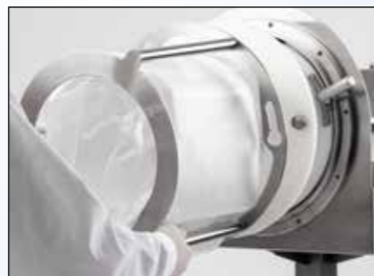
Mount the retaining basket
