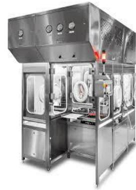
The system controls the full air flow (inlet and outlet), allowing the correct pressure to enter in the system thus making it suitable to be used with slightly toxic products. These systems cannot be used for highly toxic products. However this can be considered as the right technology to be applied when a slightly potent/toxic product is to be manipulated. Just like isolators, even closed RABS internally assure a "class A" environment, being the surrounding area classified as "class B".
